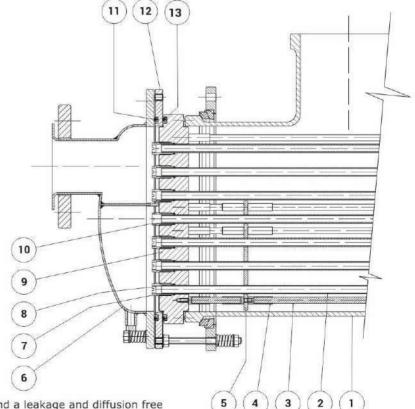
The tube sheet is the sealing part where all tubes fit, and a leakage and diffusion free partition is made between shell side and tube side. Baffles hold the tubes in place, while
