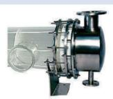
Type-II Heat exchangers are very similar to Type-I but have Metal (Mild steel or Stainless Steel) Headers instead of glass headers. These are used in applications where there is no risk of corrosion at the service/utility side. The process side comes in contact only with the glass shell or PTFE components, and hence can be corrosive. Thus, this design is generally used for condensation and tempering of corrosive liquids.
